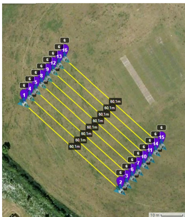
FIGURE 2 Drone's scanning pattern in a 30 m × 60 m area [52] [Color figure can be viewed at wileyonlinelibrary.com ]
