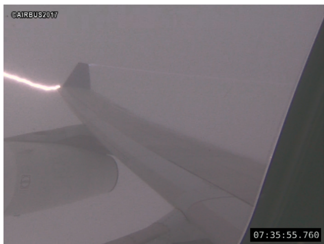
Figure 7. The video frame shows a leader channel attached to the right wing. The frame is taken at t = 07:35:55.760 UTC. A lightning leader is attached to the wing and pointed toward the nose. Ionization of the wingtip vortex is visible going along the aircraft path.
