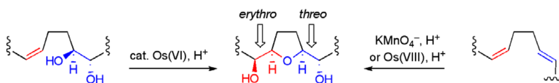
Figure 11. Synthesis of 2,5 cis -disubstituted THF diols by metal oxo mediated oxidative cyclisation.
