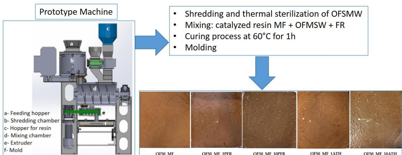
**Figure 1.** Representative scheme of the production of the experimental panels and pictures showing the top surface of each realized panel.
