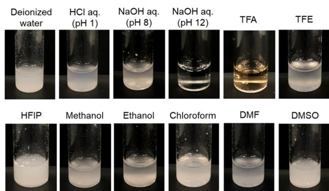
**Figure 5.** Solubility testing of the precipitated polySer (10 mg/mL). Photographs of the resultant solution after dissolving the polySer that formed during polymerization.
