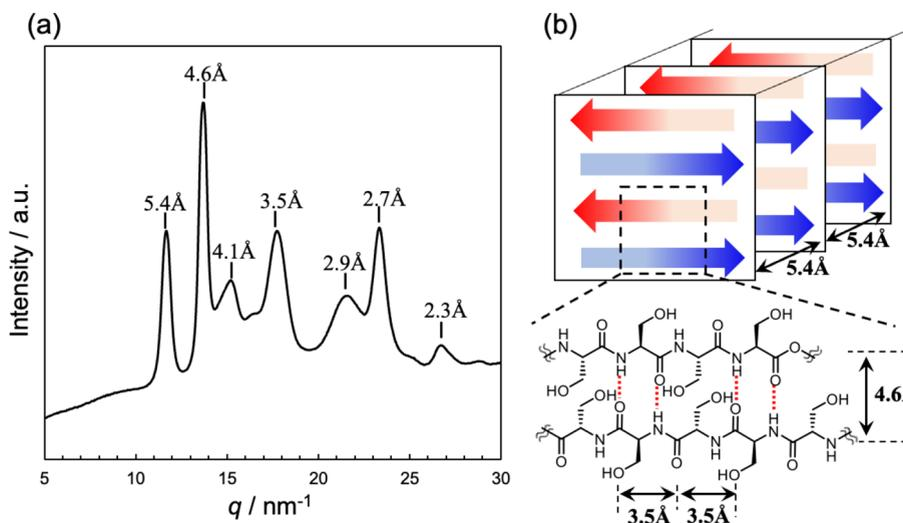
**Figure 7.** (a) 1D powder WAXD profile of polySer and (b) schematic illustration of the antiparallel  $\beta$ -sheet structure of polySer.
