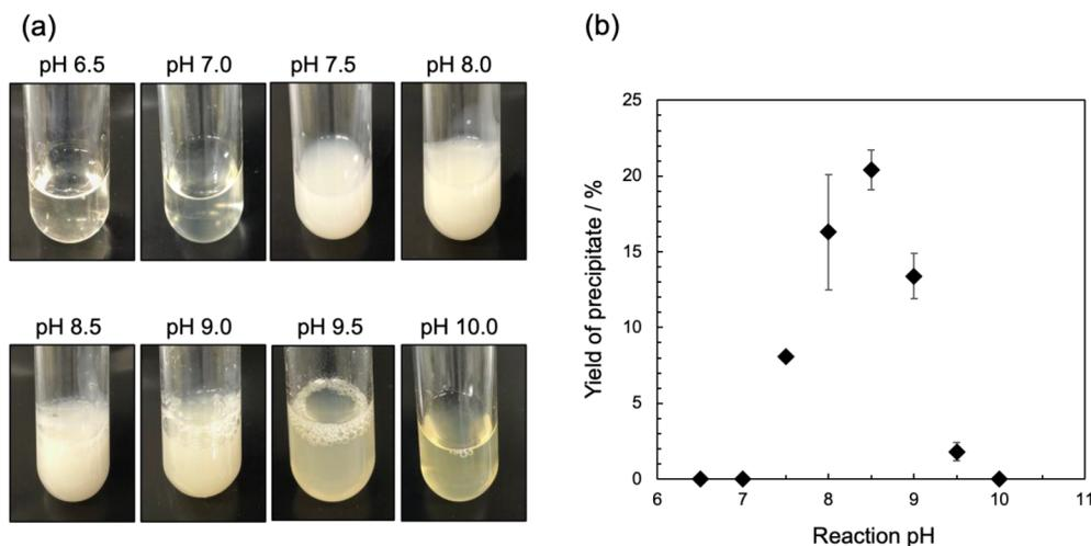
**Figure 1.** (a) Photographs of the resultant solution after the CEP of Ser-OEt at various pH conditions. (b) Yield of the precipitate formed after the CEP of Ser-OEt at various pH conditions. The precipitate was obtained as an insoluble part after washing with deionized water by the centrifugation/redispersion process to remove the remaining monomer and papain.
