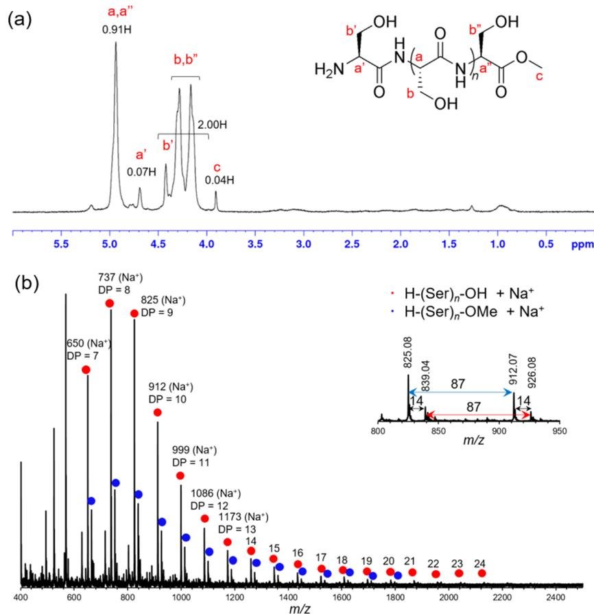
**Figure 4.** (a)  $^1\text{H}$  NMR and (b) MALDI-TOF MS spectra of the precipitated polySer obtained by the CEP of Ser-OMe at pH 8.5. TFA-*d* was used as the solvent for  $^1\text{H}$  NMR.
