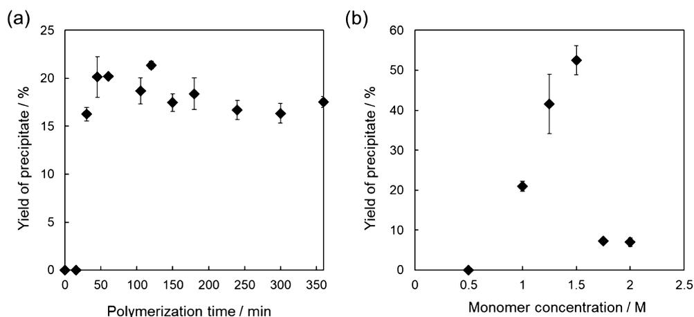
**Figure 2.** (a) Time course of the yield of the precipitate during the CEP of Ser-OEt conducted with papain (50 mg/mL) at pH 8.5. The monomer concentration was fixed at 1 M. (b) Yield of the precipitate for CEPs conducted at various monomer concentrations. The yield was an average of three independent experiments to determine the standard deviation ( $N = 3$ ).
