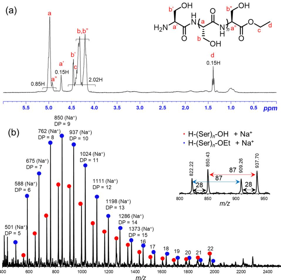
**Figure 3.** (a) <sup>1</sup>H NMR and (b) MALDI-TOF MS spectra of the precipitated polySer obtained by the CEP of Ser-OEt at pH 8.5. TFA-*d* was used as the solvent for <sup>1</sup>H NMR.
