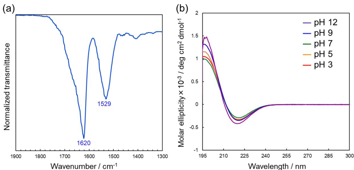
**Figure 6.** (a) IR spectrum of the precipitated polySer obtained after CEP at pH 8.5. (b) CD spectra of polySer in water at various pH values and 20 °C. The peptide concentration was 0.5 mg/mL.
