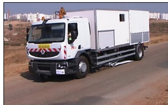
Fig. 7. Deflectograph Lacroix measurement [12].
