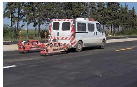
Fig. 8. Longitudinal Profil Analyzer measurement [13].
