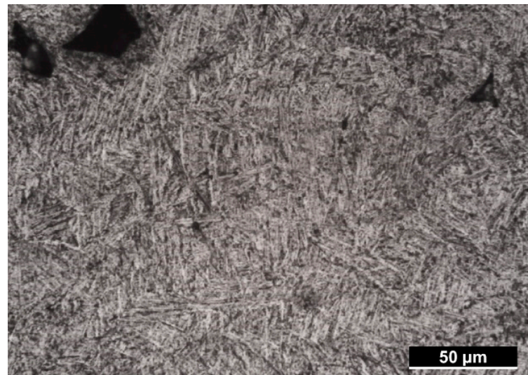
Figure 4. Representative microstructure after stress relief heat treatment. Basket weave microstructure is apparent.
