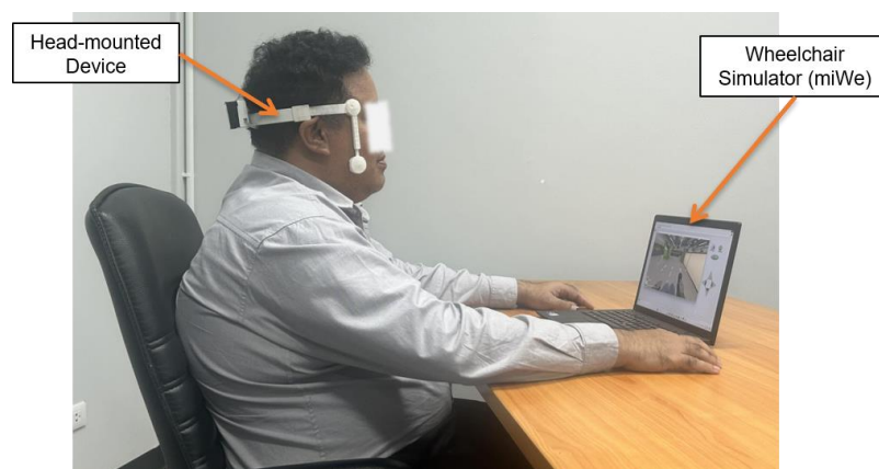
Figure 6. An example scenario of using the proposed HMIs to control a simulated wheelchair during the experiment.
