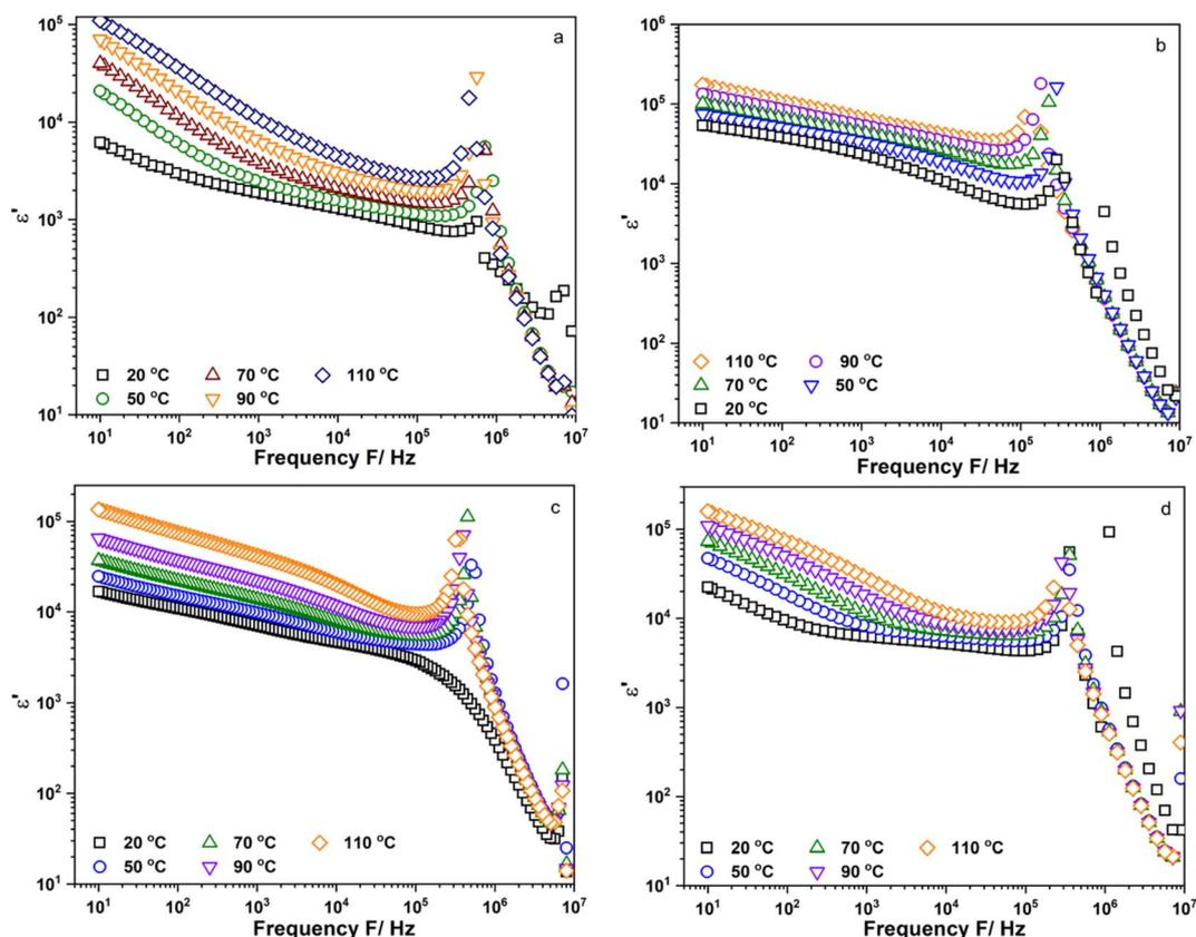
**Fig. 4** Frequency dependent of the real part of permittivity,  $\epsilon'$ , of (a)  $\text{Li}_6\text{PS}_5\text{Cl}$ ; (b)  $\text{Li}_{5.94}\text{Ca}_{0.03}\text{PS}_5\text{Cl}$ ; (c)  $\text{Li}_{5.94}\text{Mg}_{0.03}\text{PS}_5\text{Cl}$  and (d)  $\text{Li}_{5.94}\text{Al}_{0.02}\text{PS}_5\text{Cl}$  measured from 10 Hz to 9 MHz.
