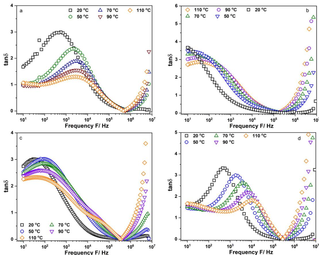
Fig. 5 Frequency dependent of the loss factor,  $\tan \delta$ , of (a)  $\text{Li}_6\text{PS}_5\text{Cl}$ ; (b)  $\text{Li}_{5.94}\text{Ca}_{0.03}\text{PS}_5\text{Cl}$ ; (c)  $\text{Li}_{5.94}\text{Mg}_{0.03}\text{PS}_5\text{Cl}$  and (d)  $\text{Li}_{5.94}\text{Al}_{0.02}\text{PS}_5\text{Cl}$  measured from 10 Hz to 9 MHz.
