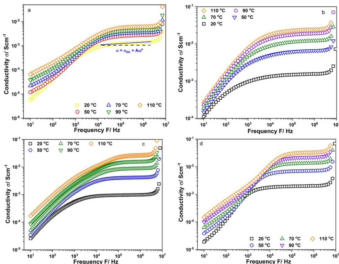
Fig. 2 Conductivity isotherms of (a) Li<sub>6</sub>PS<sub>5</sub>Cl; (b) Li<sub>5.94</sub>Ca<sub>0.03</sub>PS<sub>5</sub>Cl; (c) Li<sub>5.94</sub>Mg<sub>0.03</sub>PS<sub>5</sub>Cl and (d) Li<sub>5.94</sub>Al<sub>0.02</sub>PS<sub>5</sub>Cl measured from 10 Hz to 9 MHz.
