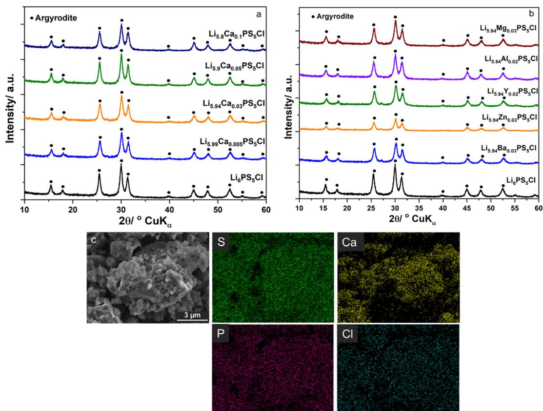
Fig. 1 Structural characterization of the prepared samples. (a) XRD patterns of  $\text{Li}_{6-2x}\text{Ca}_x\text{PS}_5\text{Cl}$  solid electrolytes; (b) XRD patterns of  $\text{Li}_{5.94}\text{M}_{0.06/n}\text{PS}_5\text{Cl}$  solid electrolytes ( $\text{M}^n = \text{Mg}^{2+}$ ,  $\text{Ba}^{2+}$ ,  $\text{Zn}^{2+}$ ,  $\text{Al}^{3+}$ ,  $\text{Y}^{3+}$ ); (c) SEM-EDS results of  $\text{Li}_{5.8}\text{Ca}_{0.1}\text{PS}_5\text{Cl}$ .
