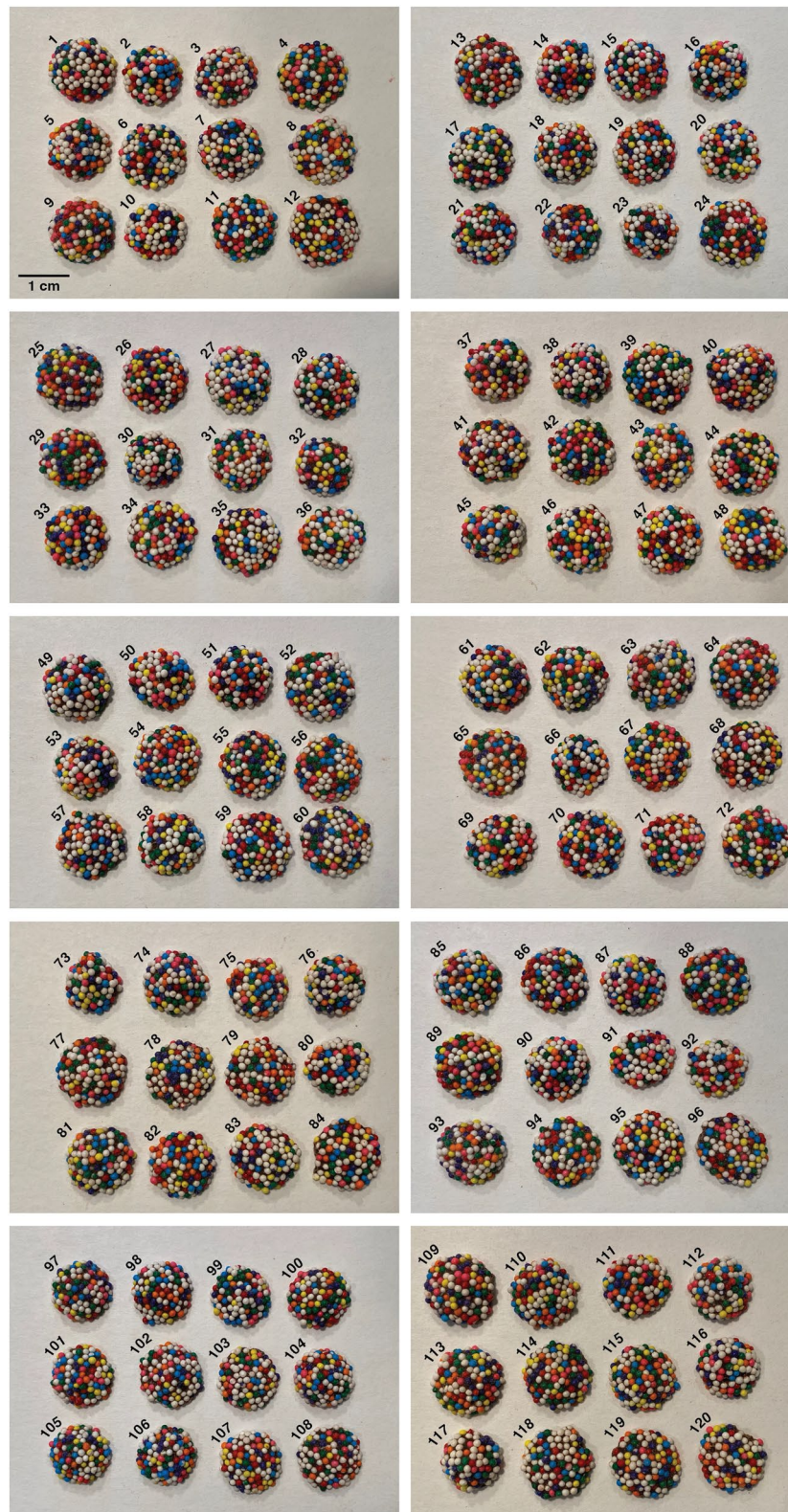
Figure 3. Photographs of 120 candies used to create a test library of CandyCodes. These commercially produced candies were used as proxies for actual CandyCoded medications. Each chocolate candy is coated by the manufacturer with an eight-color mixture of nonpareil spheres; the candies shown here received between 72 and 108 nonpareils each, with an average of 92.6 nonpareils per candy. Each CandyCode photo was converted to a set of strings using the process described in Fig. 4 and analyzed to determine its uniqueness. Additionally, three of these CandyCodes (numbers 103, 104, and 109) were selected at random and subjected to one week of physical abuse to determine if mechanical wear sustained during shipping could affect the information content of CandyCodes.
