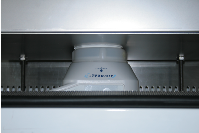
Figure 3: Position of the microbial air sampler at the opening on the bottom of the box containing the laptop
