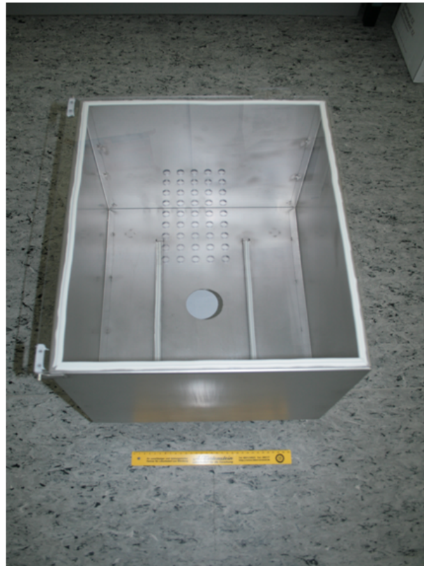
Figure 2: The metal box (which could be disinfected) and its perforated Plexiglas cover which facilitated circulation of the surrounding laminar air flow. The opening on the bottom of the box was the location where the microbial air sampler was securely joined.
