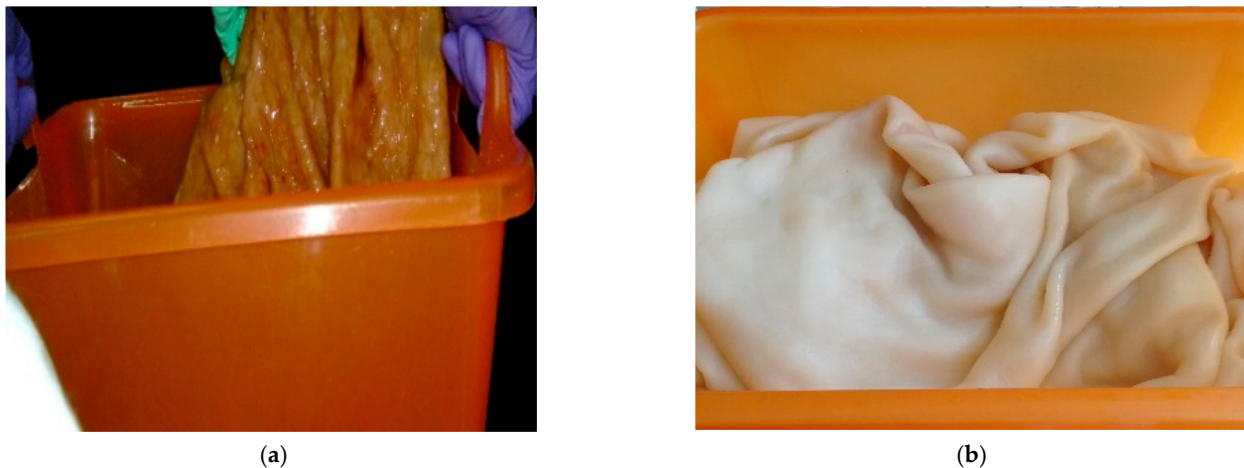
Figure 2. Washing of BNC sheets: (a) unwashed BNC sheet and (b) washed BNC sheet.
