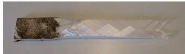
Figure 10. Failure of tension shear specimen.
