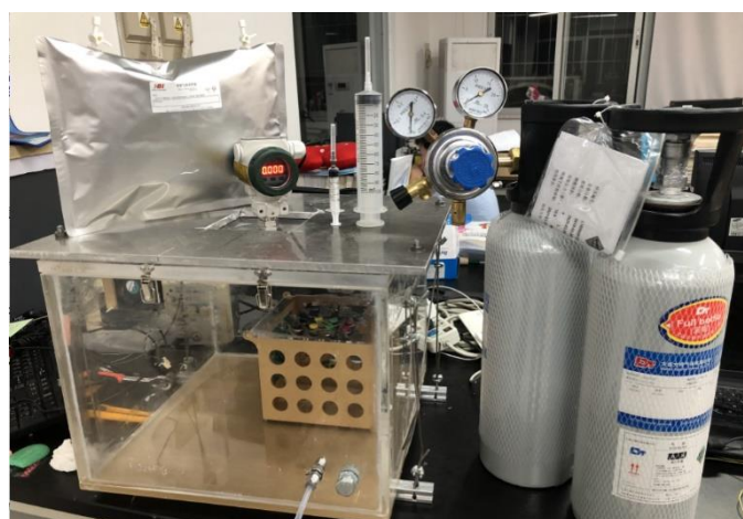
Figure 9. Photo of the air-tight chamber.
