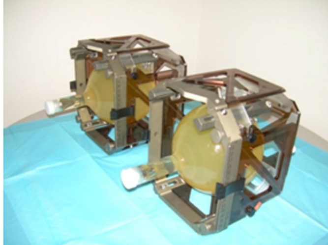
FIG. 1. Phantoms fixed in Leksell frame with indicator box for MRI scanning.
