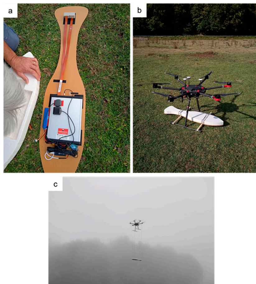
Figure 1. (a) Arrangement of the GEOMETRICS MFAM “Development kit” magnetometer inside the bird; (b) first flight configuration (F0.5), with the magnetometer fixed to the UAV landing sled, 0.5 m below the platform; (c) second flight configuration (F3.0), with the magnetometer suspended 3 m below the UAV.
