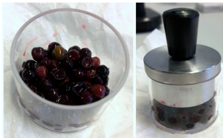
Figure 2. Elderberries compressed for near-infrared (NIR) measurements.
