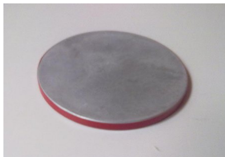
FIG. 1(c). Shielding disc (double-layered): the first being aluminum 4 mm thickness, the second comprised of 2 mm thick lead. Disc diameter is 120 mm.
