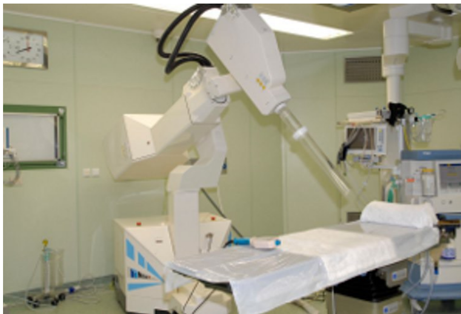
FIG. 1(a). The mobile linear electron accelerator NOVAC7 in the operating theatre.
