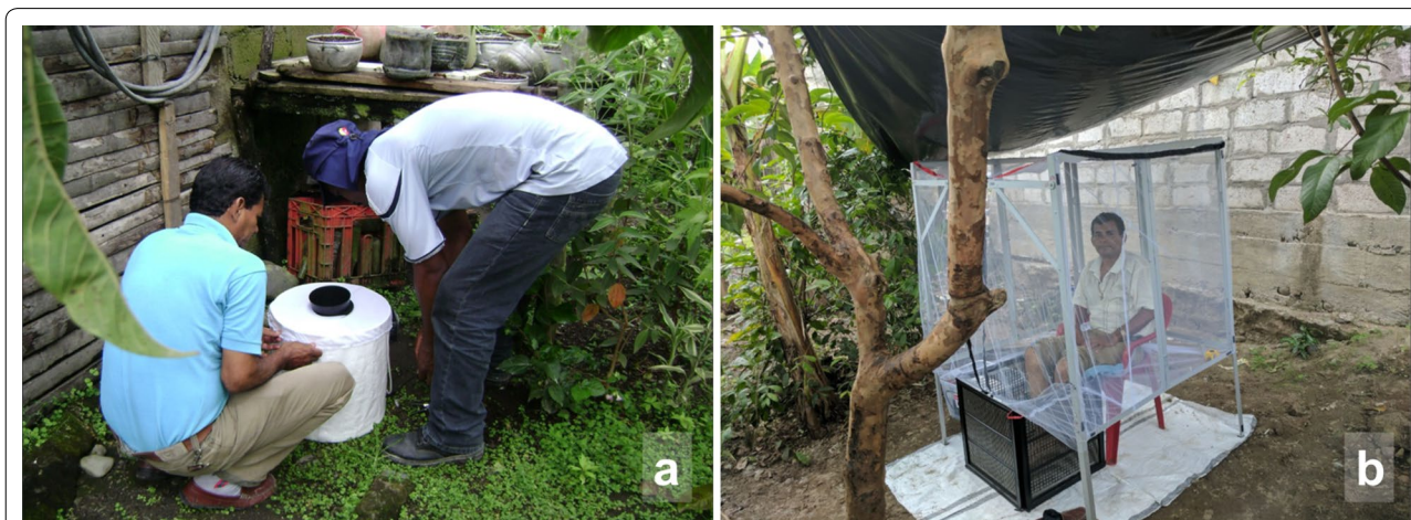
Fig. 2 Trapping methods used in this study. a Typical set-up of a BGS trap. b Set-up of a MET with a technician luring mosquitoes
