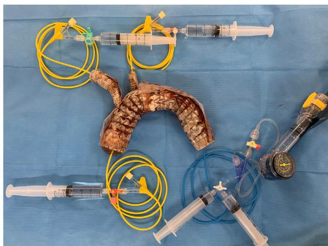
**Supplementary Fig 2.** Setup for the leak test. All outlets of the stent grafts (SGs) were blocked with Coda balloons (Cook Medical Inc) or Reliant balloons (Medtronic, Santa Rosa, CA).
