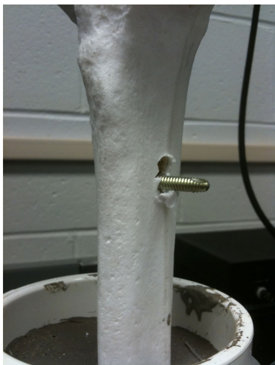
Figure 4 Failure of the distal interlocking screw at the tibia observed with axial load. This is the primary mode of failure in all tested constructs.
