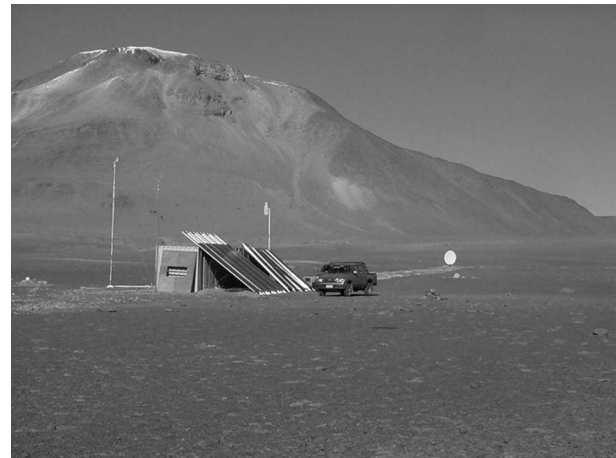
Fig. 12. (Color online) Site testing instruments and containers at the 4800 m site of Pampa la Bola. Two containers are equipped with solar panels and one of the element antennas of the radio seeing monitor can be seen in the background. (Credit: NAOJ).
