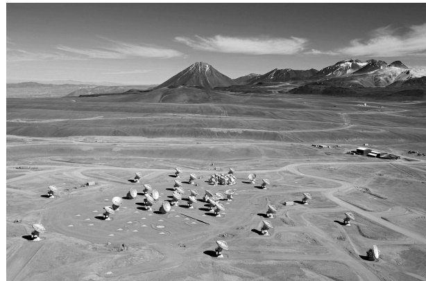
Fig. 8. (Color online) Aerial view of the central part of ALMA. Some of the empty pads for relocation are visible. Located in the center is the 7 m antennas of ACA. The building to the right is the Technical Building of the Array Operations Site. (Credit: Clem & Adri Bacri-Normier (wingsforscience.com)/ESO).
