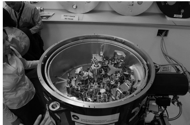
Fig. 26. (Color online) Receiver dewar that accommodates receiver cartridges and a GM cryocooler (Credit: NAOJ).
