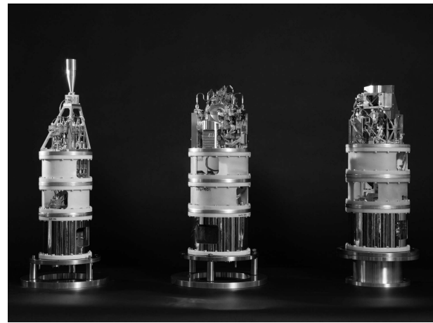
Fig. 22. (Color online) Band 4, Band 8, and Band 10 receiver cartridges (from left to right) developed by NAOJ (Credit: ALMA (ESO/NAOJ/NRAO)).
