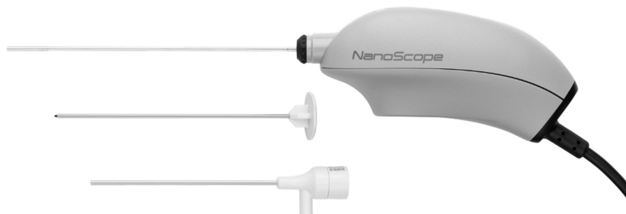
Fig 2. The needle arthroscopic device (NanoScope; Arthrex) is a needle arthroscopy device with a 1.9-mm scope. Technical characteristics: 400 × 400 resolution, 120-degree field of view, auto-focus from 3 mm × 100 mm. The device has a zero-degree viewing angle.
