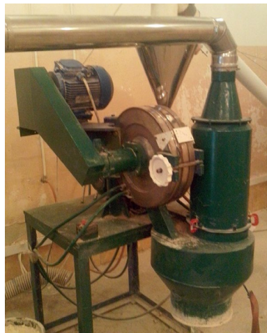
Figure 4. Appearance of the disintegrator: 1—loading funnel, 2—working chamber with grinding disks, 3—unloading hole, 4—filter, 5—electric motor.
