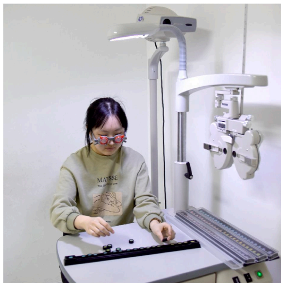
Fig. 2. Photograph of the test setup. BBLs or control lenses were inserted into the forwardmost cells, while correct lenses were inserted into the rearmost cells of the trial frame.
