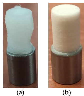
Figure 7. Obtained prints: (a) deformed PA overprint on a sample that was not cooled down after three layers were applied; (b) correctly printed PLA overprint.
