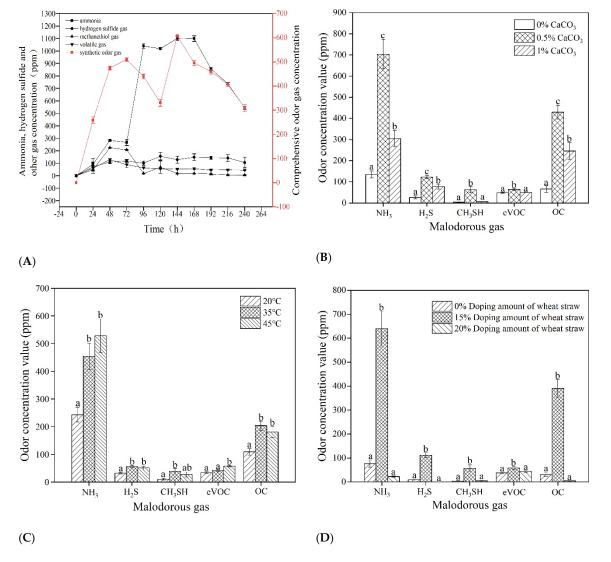
adding 0% calcium carbonate and 20% wheat straw at the temperature of 20  $^{\circ}$ C, the odor production is the least on the second day and long-term stacking of pig manure should be avoided as far as possible.
