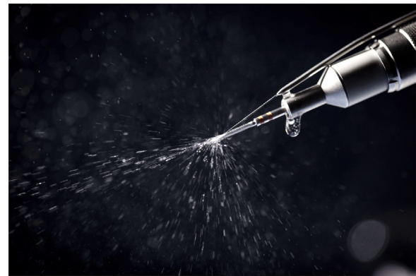
Fig. 1. Still photograph of aerosol generation from a standard handpiece with inbuilt irrigation at 60000 RPM.
