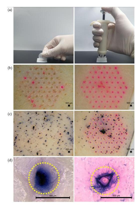
**Figure 3.** Analysis of the skin penetration of TA-DMNs applied using a shooting device or finger force: (**a**) TA-DMN patches application performed using finger force or a shooting device; (**b**) porcine skin inserted with Rhodamine B-loaded TA-DMNs using a finger force or a shooting device; (**c**) verification of porcine skin penetration by trypan blue staining; (**d**) enlarged images of perforated porcine skin. The black bar represents 500 μm.
