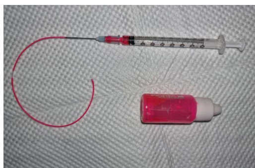
Figure 1. Tattoo ink and a customized instrument for ink placement. The customized instrument is a PTFE Teflon tube with 0.5 mm inner diameter and 0.9 mm outer diameter attached to a 1 mm syringe.
