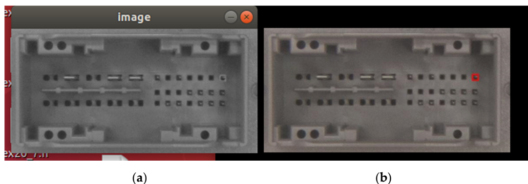
Figure 9. OPC UA publish–subscribe, 20-channel image transmission for ECU automatic optical inspection process in the automotive manufacturing: (a) the received image and (b) the target image.
