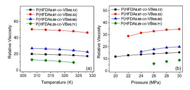
Figure 7. Relative viscosities of the co-polymer–CO<sub>2</sub> systems versus temperature (a) and pressure (b).
