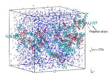
**Figure 2.** Optimized conformation of the polymer–CO<sub>2</sub> system (CO<sub>2</sub> was marked as blue line molecular; while polymer chain was marked as ball and stick figure).
