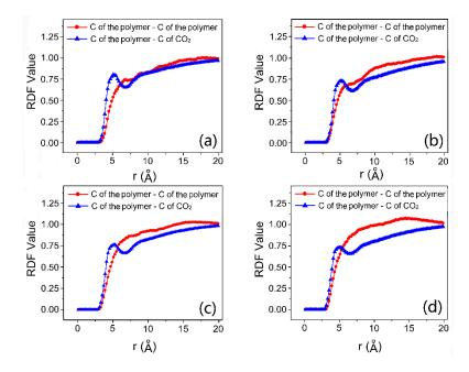
**Figure 5.** Intermolecular RDFs of the carbon-carbon pairs of polymer–polymer and polymer–CO<sub>2</sub>. (a) P(HFDA<sub>0.87</sub>-*co*-VBe<sub>0.13</sub>); (b) P(HFDA<sub>0.67</sub>-*co*-VBe<sub>0.33</sub>); (c) P(HFDA<sub>0.50</sub>-*co*-VBe<sub>0.50</sub>); (d) P(HFDA<sub>0.29</sub>-*co*-VBe<sub>0.71</sub>).
