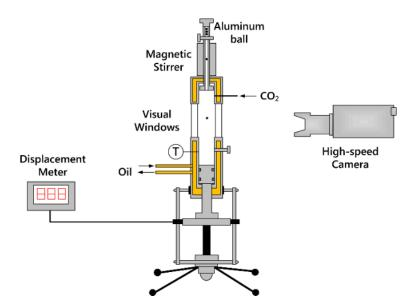
**Scheme 2.** High-temperature and high-pressure visual unit used for cloud point and viscosity measurements.
