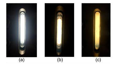
**Figure 1.** The phase transitions of supercritical  $CO_2$ -polymer system under constant temperature, (**a**) single phase (above cloud point); (**b**) the appearance of the mist (cloud point); and (**c**) two phase (below cloud point).
