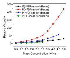
**Figure 6.** Relative viscosities of the co-polymer–CO<sub>2</sub> systems at 308.2 K and 30 MPa versus mass concentration.
