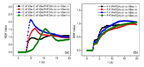
**Figure 9.** Radial distribution functions of the intermolecular C-C pairs of VBe groups (**a**) and F-F pairs of HFDA groups (**b**).
