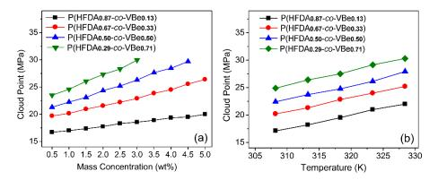
**Figure 4.** Cloud point pressures of the co-polymer– $CO_2$  solutions versus mass concentration at 308.2 K (a) and temperature (b) at 1 wt. % of concentration.
