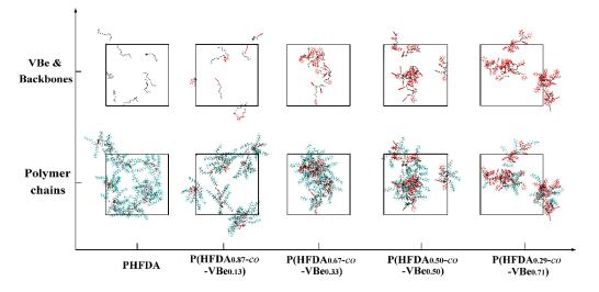
**Figure 8.** Equilibrium conformations of five CO<sub>2</sub>–polymer systems at 308.2 K and 25 MPa. All the CO<sub>2</sub> molecules were deleted to highlight the polymer chains (**lower**) and the specific functional groups and backbones (**upper**).
