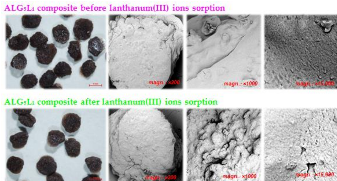
Figure 2. OM and SEM images of ALG 5 L 1 composite before and after La(III) ions sorption at a magnification of 200, 1000, and 15,000 \times .
