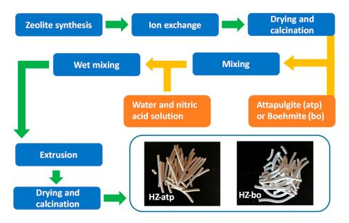
**Figure 1.** Steps in the preparation of zeolite extrudates with attapulgite and boehmite and key sample photos.
