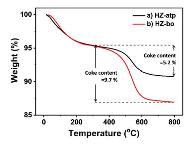
**Figure 8.** Thermogravimetric analysis (TGA) curves of HZ-atp (black) and HZ-bo (red) after toluene methylation reaction. Coke content was calculated by ([mass of 300 °C] – [mass of 800 °C])/[mass of 800 °C] × 100%.
