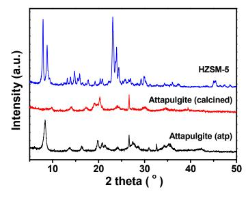
**Figure 2.** X-ray powder diffraction (XRD) patterns of H-ZSM-5 powder; the attapulgite binder before and after calcination
