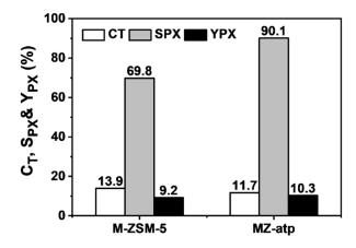
**Figure 11.** Toluene conversion, para-selectivity and yield of para-xylene over modified ZSM-5 (M-ZSM-5) and its extrudate with attapulgite (MZ-atp). Reaction conditions: 460 °C, atmospheric pressure, WHSV =  $15 \text{ h}^{-1}$ , nT/nM = 4,  $\text{nH}_2/\text{n}(\text{T} + \text{M}) = 2$ ,  $\text{nH}_2\text{O}/\text{n}(\text{T} + \text{M}) = 2$ .
