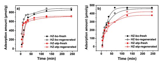
Figure 10. n-Hexane (a) and cyclohexane (b) adsorption of fresh and generated zeolite extrudates.
