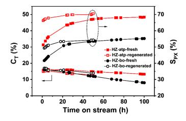
**Figure 7.** Toluene conversion and para-selectivity as a function of time on stream over HZ-atp (square) and HZ-bo (circle). Solid for fresh catalysts and open for regenerated catalysts.
