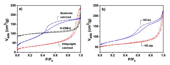
Figure 5. Nitrogen adsorption/desorption isotherms of powders (a) and extrudates (b).
