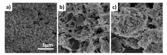
**Figure 4.** Scanning electron microscopy (SEM) images of H-ZSM-5 (**a**), attapulgite (**b**) and calcined HZ-atp extrudate (**c**). The scale bar represents 1 µm and applies to all images.
