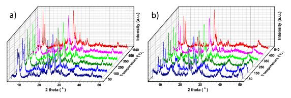
**Figure 3.** In situ XRD patterns of HZ-atp (**a**) and HZ-bo (**b**); in situ scanning at 100 °C steps from 50 °C to 540 °C under synthetic air.
