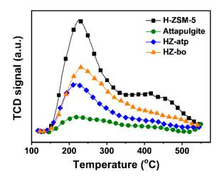
Figure 6. NH<sub>3</sub>-TPD profiles of H-ZSM-5 zeolite and HZ-atp and HZ-bo extrudates.
