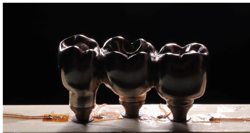
Figure 11. Positioning of four strain gauges on the surface of a polyurethane block.
