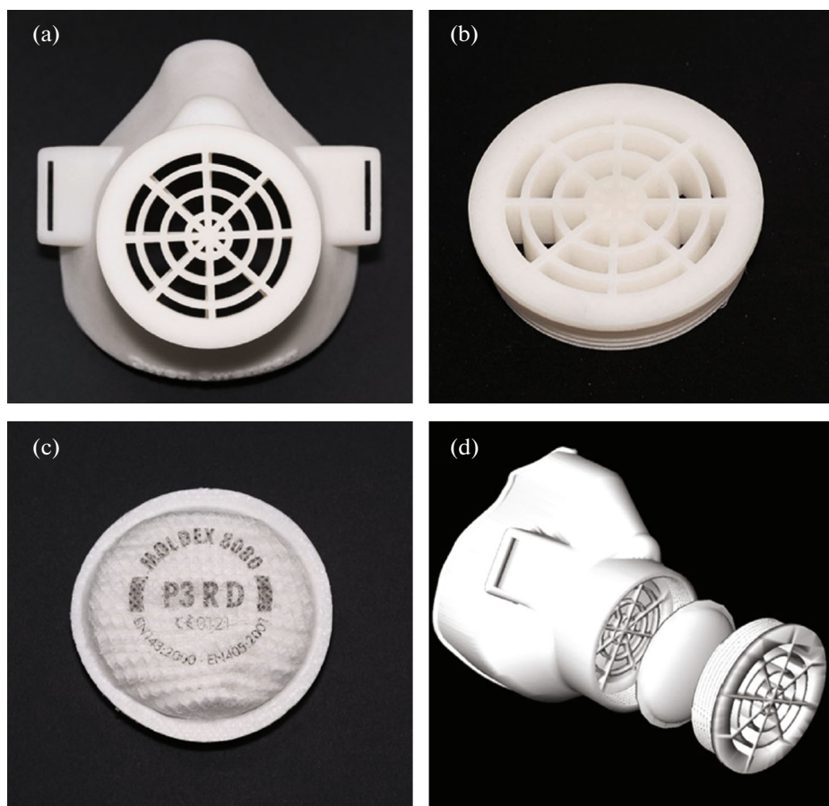
Fig. 12. (Color online) Individualized RPE obtained by 3D printing: (a) reusable half-mask, (b) support for a filtering membrane, (c) filter from polypropylene-based nonwoven material, and (d) 3D image of the prototype [1].
