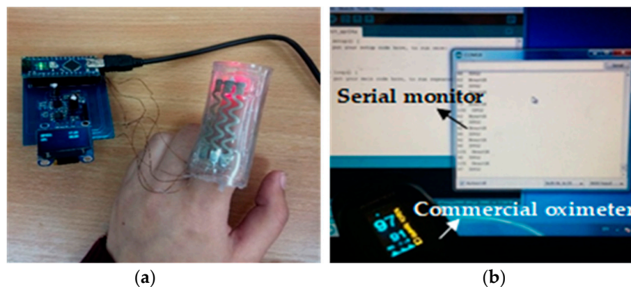
Figure 20. Functional stretchable pulse oximeter. (a) The stretchable pulse oximeter is interfaced with external circuitry; (b) data is collected by the sensor displayed on Arduino serial monitor and sensor output is compared to a commercial pulse oximeter.
