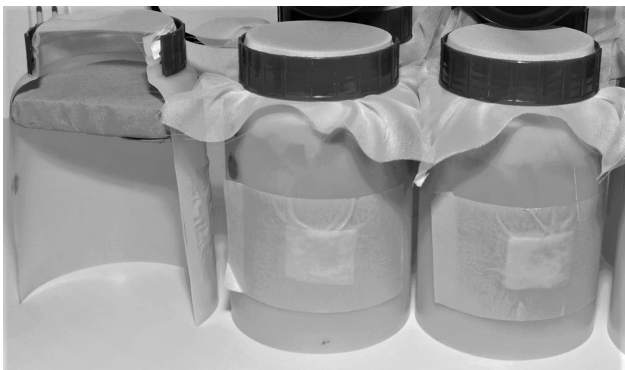
Picture 1. Feeding pots—specially designed containers used during infection feeding of sand flies conducted in BSL3 facilities.
