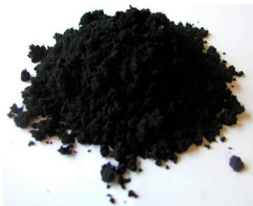
Figure 1. Photograph of multi-walled carbon nanotubes (MWCNTs) powder obtained by mechanical grinding of macro cylinders with walls consisting of radially oriented MWCNTs.
