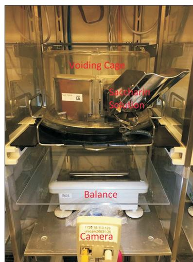
**Fig. 1.** Voiding cage. Metabolic cage and rat grid floor with access to saccharin solution, above sensitive balance. Session recording by high definition camera.
