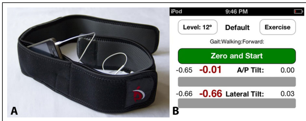
Figure 2. Level Belt. The Level Belt is a commercialized iPod application and lumbopelvic belt setup that measures anterior/posterior and medial/lateral tilt during functional activities. A, Level Belt setup with iPod in pocket. The belt is placed over bilateral anterior superior iliac spines and the iPod is centered in the midline of the patient’s spine. B, Example screen of data capture using the Level Belt iPod application.
