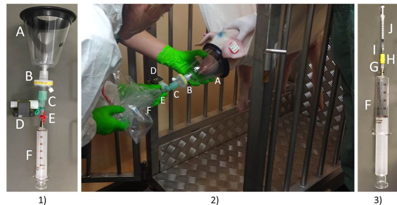
Figure 5. Breath sampling under high safety conditions. (1) breath sampling device, (2) breath sampling from swine in canvas sling, and (3) bi-directional NTD-sampling. A = breathing mask, B = virus-bacteria filter, C = T-piece, D = capnometer, E = three-way cock, F = 50 ml glass syringe, G = female/female adapter, H = IN stopper, I = Needle-trap, J = 1 ml syringe.
