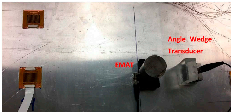
Figure 12. Experimental setup for modal decomposition. An angle wedge transducer and EMAT are used to generate mixed wave simultaneously.
