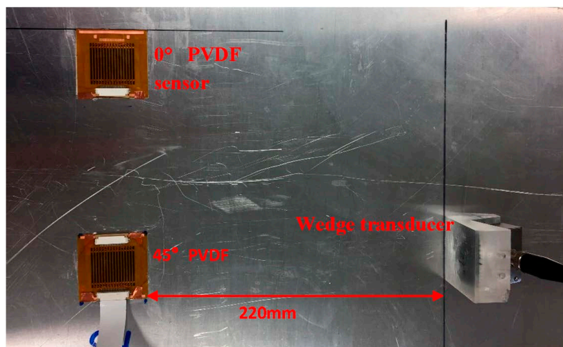
Figure 8. Experimental setup for PVDF sensors to receive Lamb waves.
