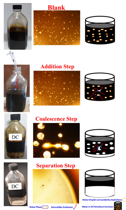
Figure 12. Microscopic inspection of the demulsification mechanism.
