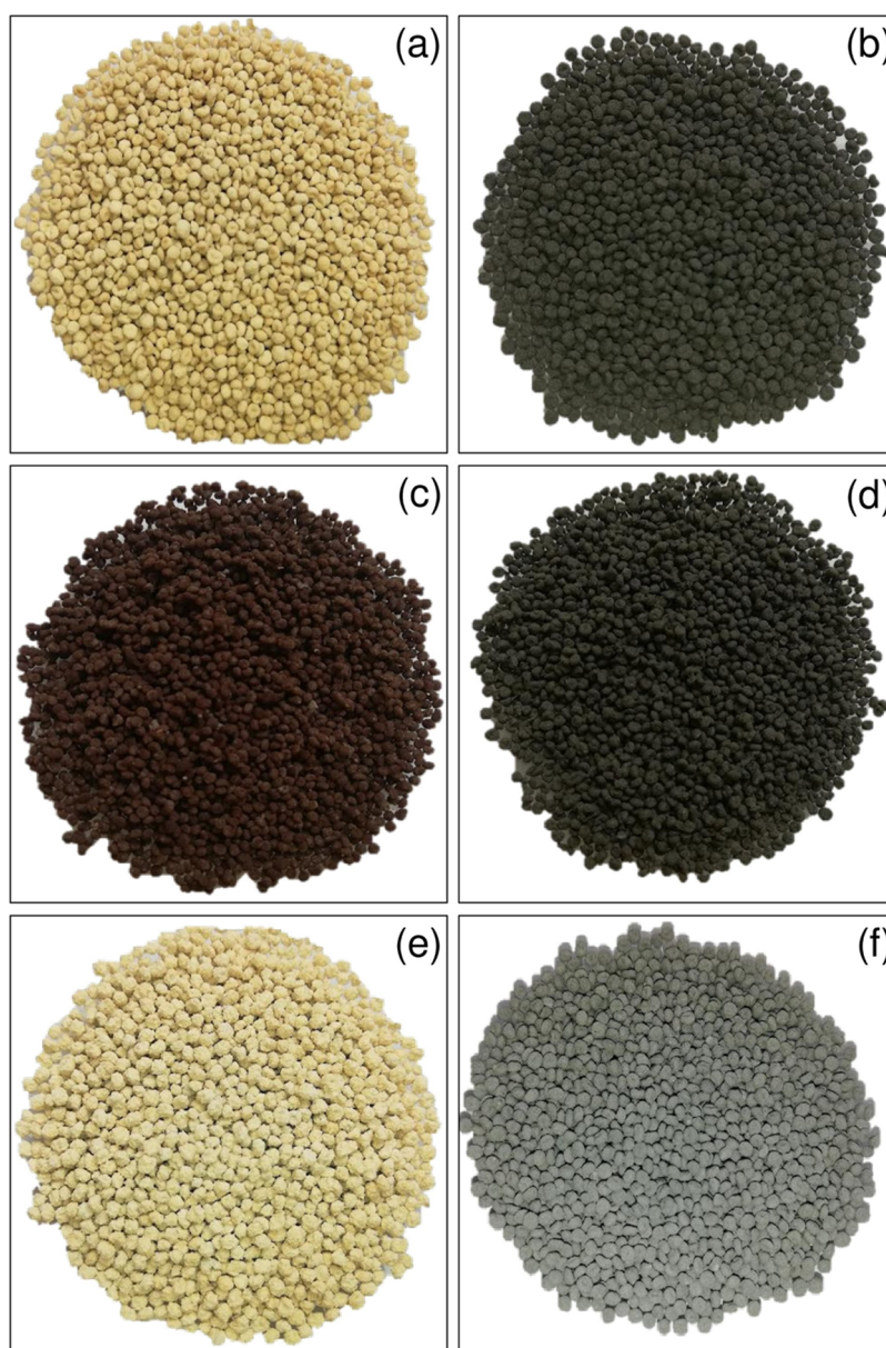
Figure 1. Physical characteristics of (a) bagasse beads (BB), (b) bagasse fly ash beads (BFB), (c) bagasse beads with mixed iron(III) oxide-hydroxide (BBF), (d) bagasse fly ash beads with mixed iron(III) oxide-hydroxide (BFBF), (e) bagasse beads with mixed zinc oxide (BBZ), and (f) bagasse fly ash beads with mixed zinc oxide (BFBZ).
