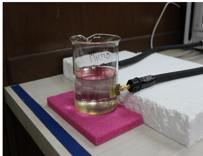
Figure 15. Measurement setup of the proposed UWB antenna sensor.
