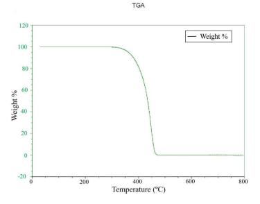
Figure 5. Thermogravimetric analysis of PP.
