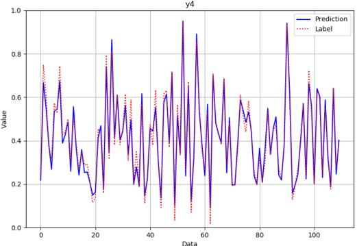
**Figure 15.** Comparison of predicted and actual values in the modulus of resilience verification data set after normalization.
