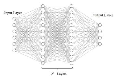
Figure 7. The architecture of the neural network.
