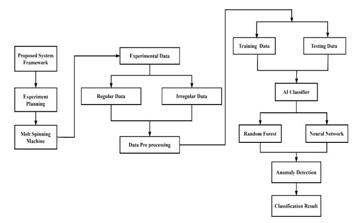
Figure 1. Flowchart for anomaly detection.
