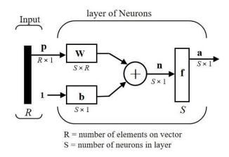
Figure 2. Single-layer neural network architecture.
