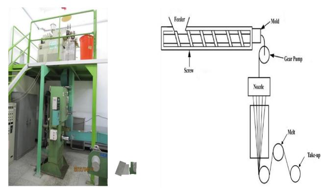
Figure 4. Melt spinning machine process.
