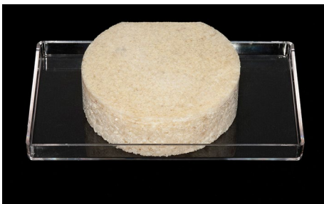
FIGURE 1 Standardised bovine bone specimen (BoneSim, 1800.35/1300.14 Composite, BoneSim, Newaygo, MI, USA) embedded in polystyrene test box
