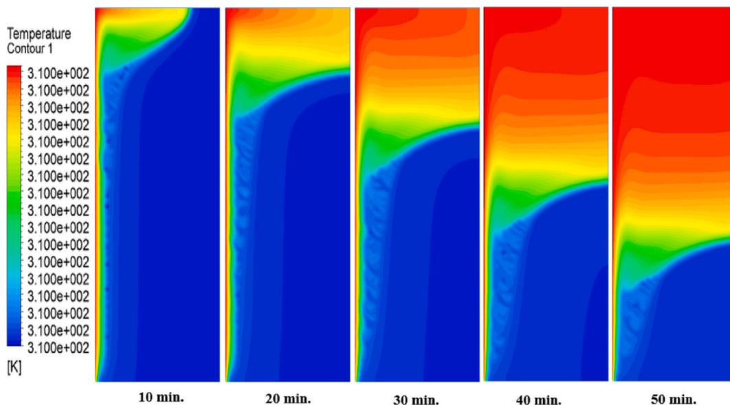
Fig. (4). Temperature distributions without fins.
