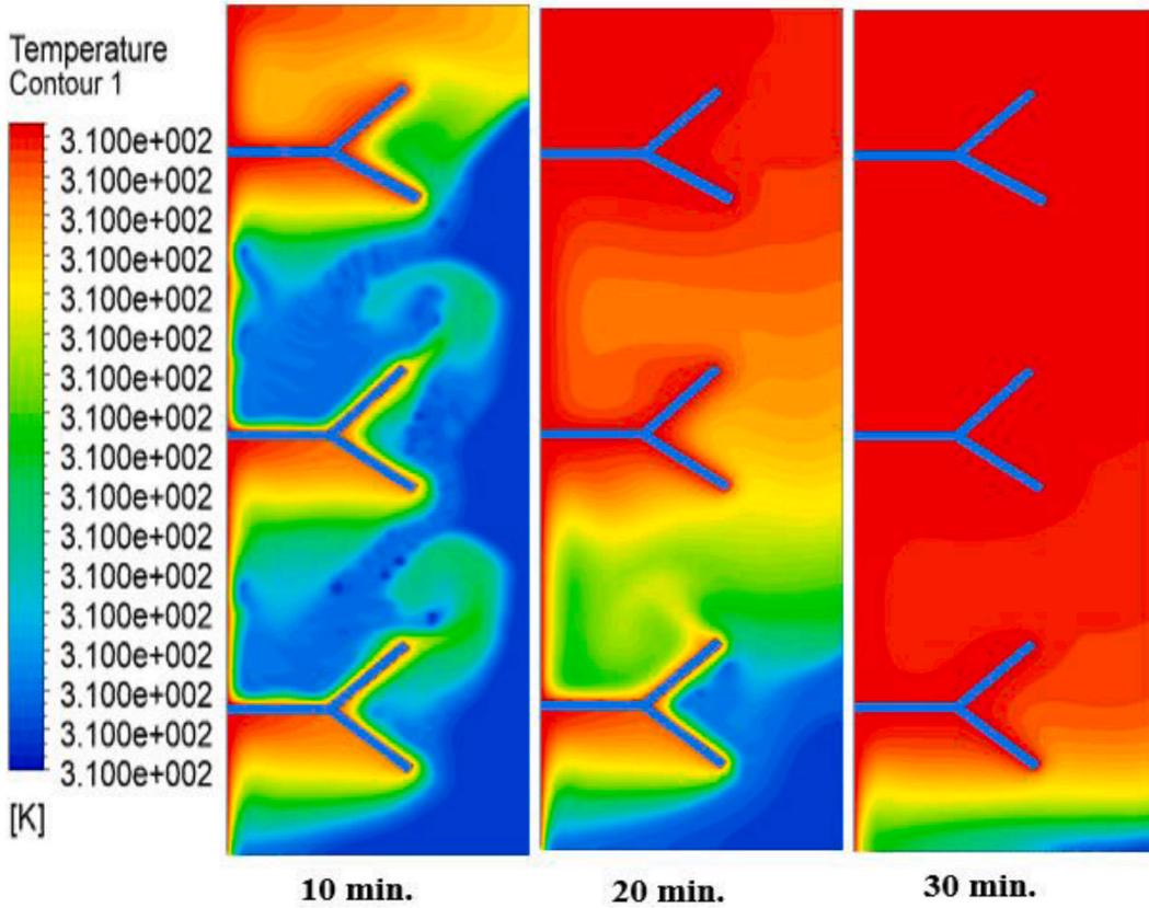
Fig. (10). Temperature distributions with three v-shaped fins.
