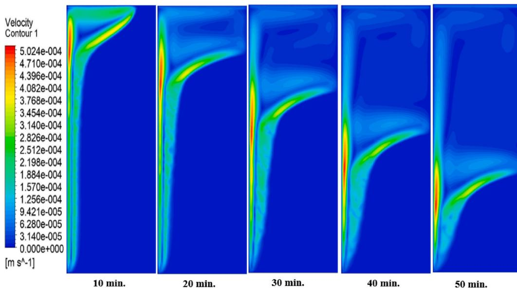
Fig. (5). Velocity distributions without fins.
