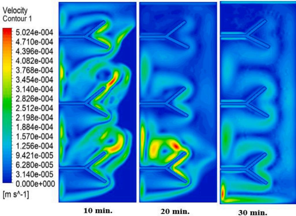
Fig. (11). Velocity distributions with three v-shaped fins.
