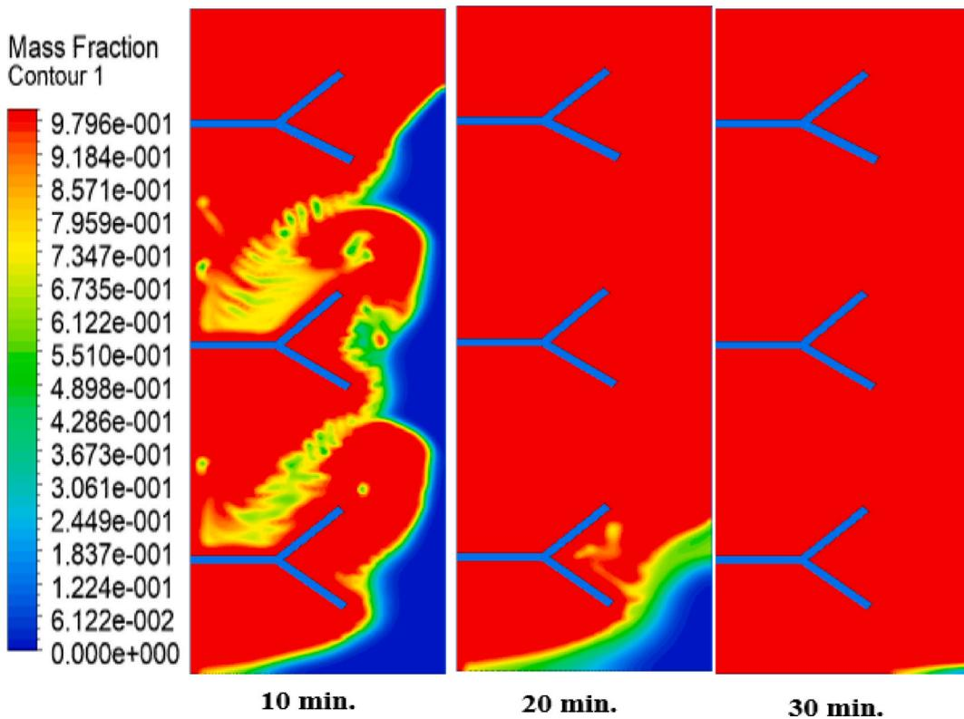
Fig. (9). Predicted evolution of the melting process with three v-shaped fins.
