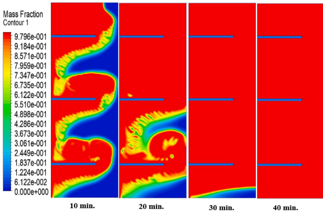
Fig. (6). Predicted evolution of the melting process with three fins.
