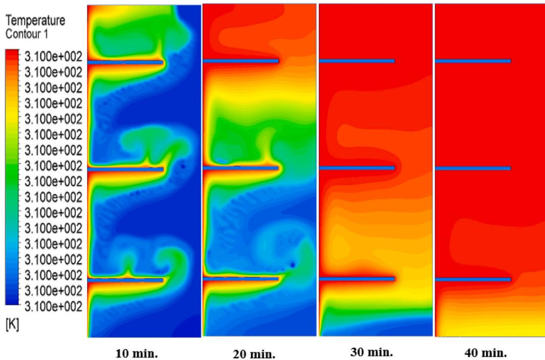
Fig. (7). Temperature distributions with three fins.
