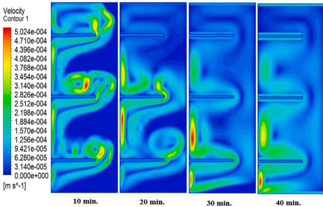
Fig. (8). Velocity distributions with three fins.
