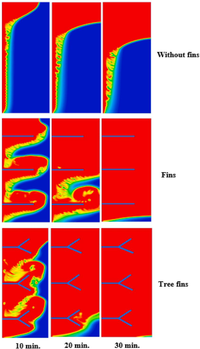
Fig. (12). Comparison of the melting process between all cases.
