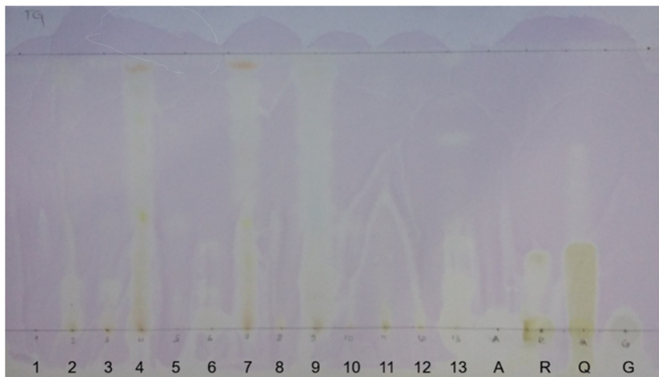
Figure 6. Qualitative analysis of antioxidant activity using thin layer chromatography (TLC). 20×20 alumina TLC plate showing yellow bands of all fungal extracts and standards: Ascorbic acid (A), Rutin (R), Quercetin (Q) and Gallic acid (G) after spraying with 10% \text{AlCl}_3 solution followed by 0.04% DPPH solution.
